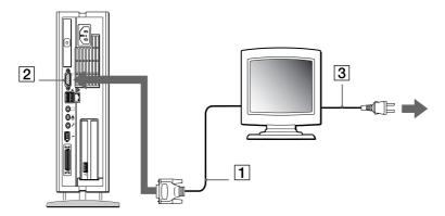
Do not turn the power on, either on the computer or the new monitor, until all connections are in place.
